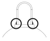
Make sure the click mechanism, on both sides, is anchored to the top of the lantern.
